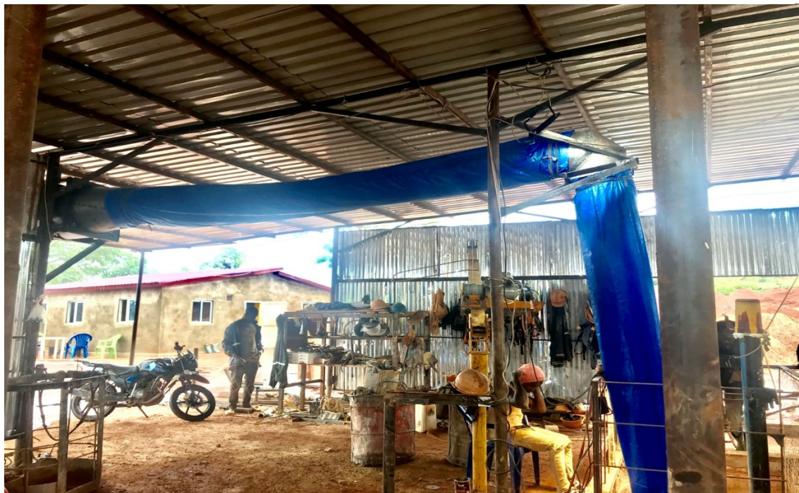
Figure 2.5 Air supply system
