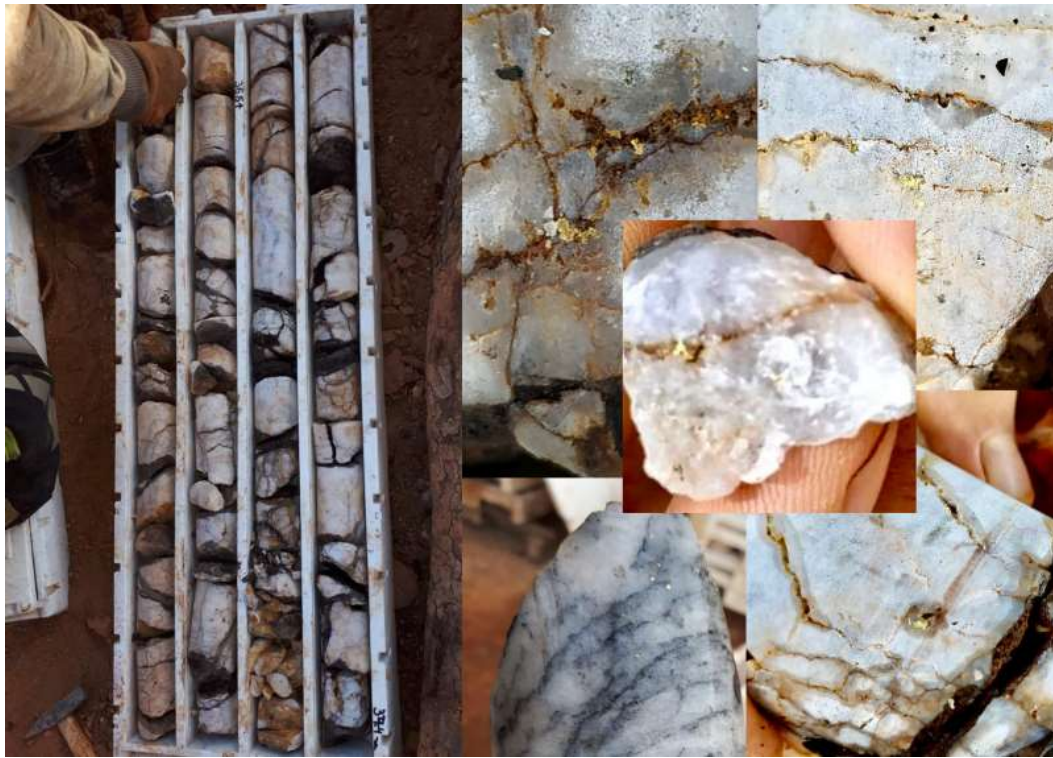
Figure 16 – Quartz ore obtained after diamond drilling. Gold kernels are visible upon inspection
